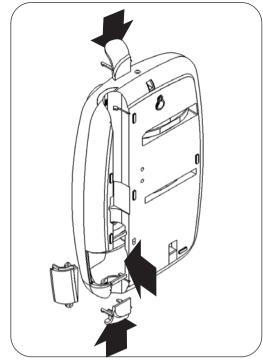
We have incorporated into the bottom right-hand side of the back plate an easy removable trim section, to allow easy access when connecting the water supply. (*Please Note!* Remember to replace this trim section before refitting the cover).
