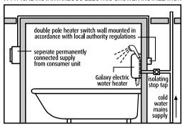
Plan your own installation carefully. Check on the nearest and most readily accessible rising mains water supply, this may be beneath the bath or in the loft, where it feeds the cold water storage tank. Use only the cold rising water main supply. Do not connect the shower unit to the down service from the tank.
